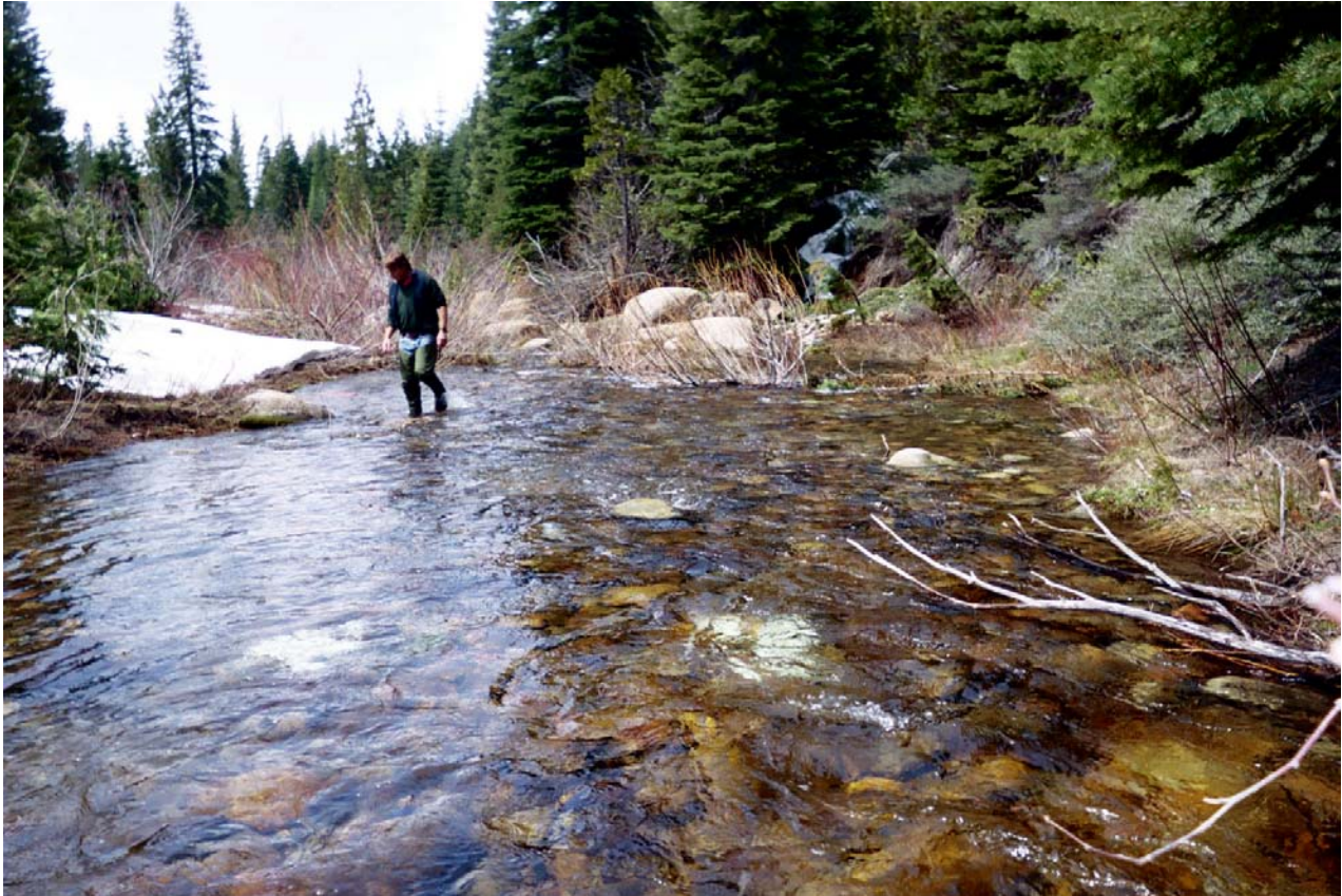
Photo 7. Upper Study Site 7 on high gradient riffle. Two white “patches” visible on the left of the photograph indicate the tracer gravels placed on the bed to track movement downstream toward the small boulder about 20 ft downstream, and the boulders visible in the center of the channel, about 50 ft downstream.
