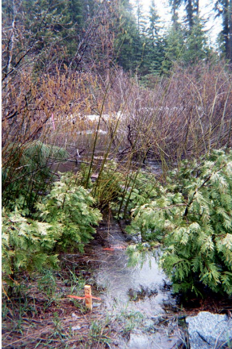
Photo C-6. Water surface elevation at Site 2, Lower Study Site, during 794 cfs flow release. Wood stake marks the water surface elevation.
