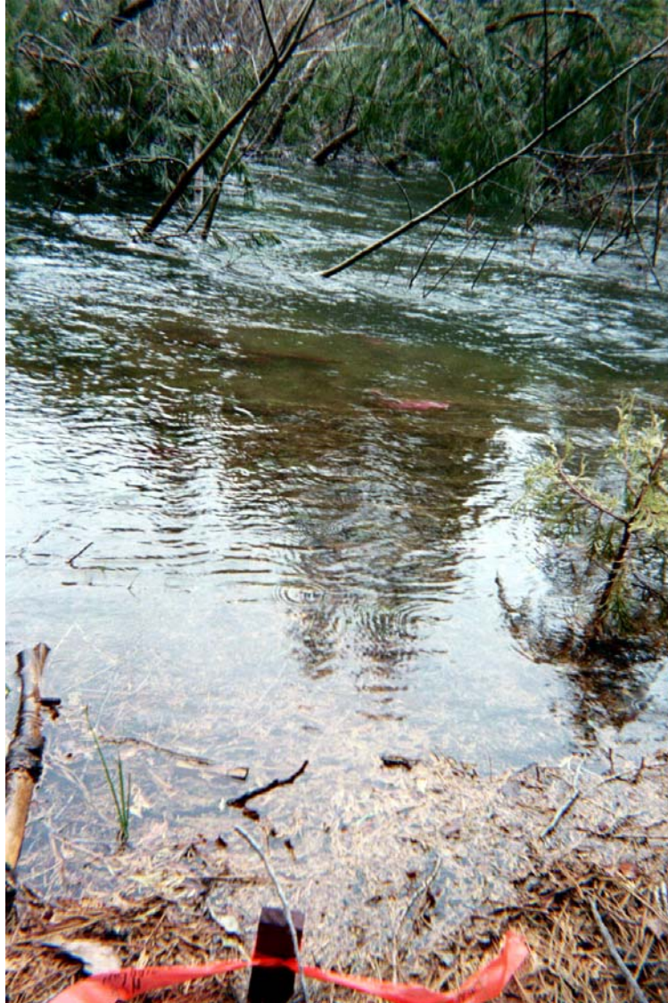
Photo C-3. Water surface elevation at Site 1, Lower Study Site, during 794 cfs flow release. Wood stake at bottom of photograph marks the river stage.
