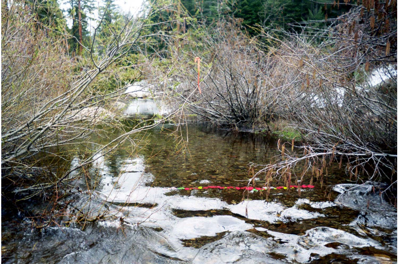
Photo 10. Lower Study Site 4. The tracers are arrayed in a cross-section line at the riffle crest (view upstream).
