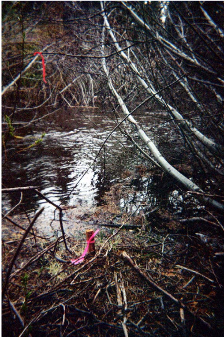
Photo C-1. Water surface elevation at Site 1, Lower Study Site, during 314 cfs flow release. Wood stake near bottom center of photograph marks the river stage, which is slightly below the rooted elevation of nearby willows.
