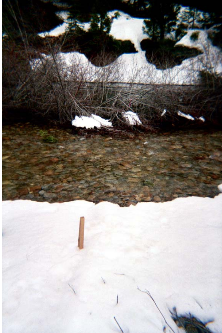
Photo C-8. Water surface elevation at Site 1, Upper Study Site, during 481 cfs flow release. Wood stake in snow marks the water surface elevation (flow has undercut snow bank on bar, not visible in photograph). Note the water surface elevation is well above the existing line of willows at edge of bar.
