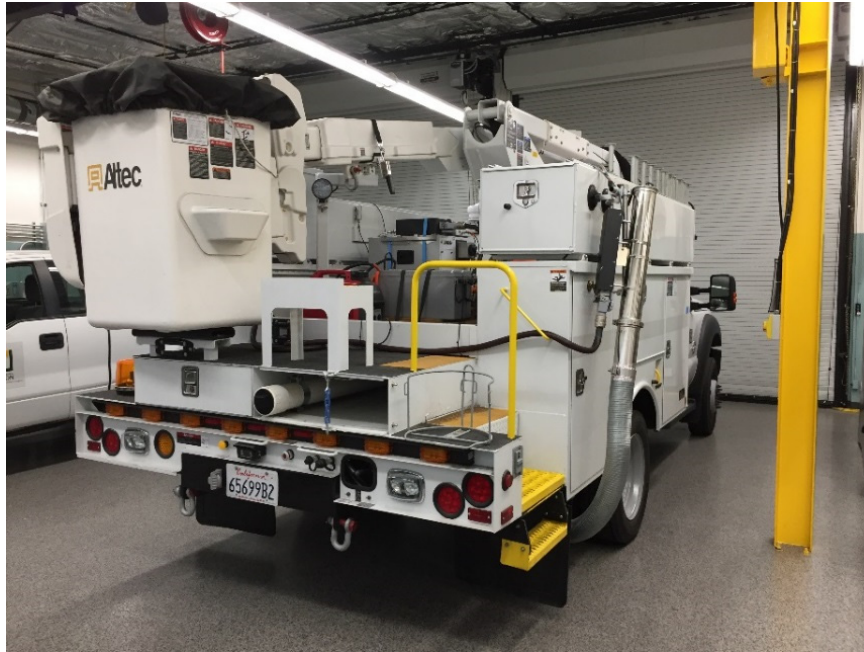
Figure 4. Rear View of AT-40 Troubleman Truck Equipped With JEMS System
