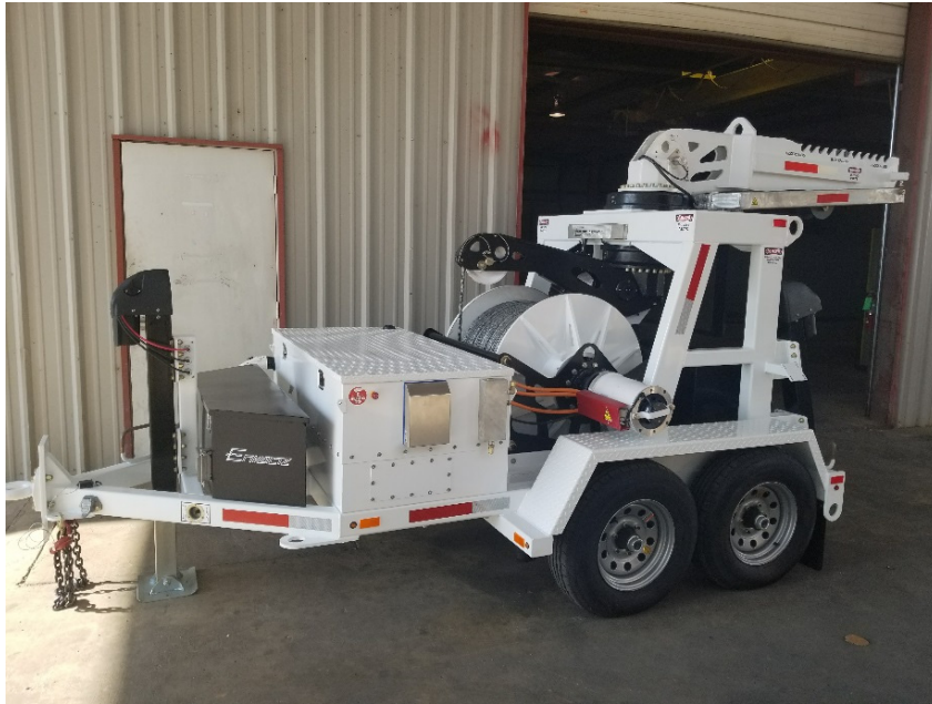
Figure 7. Envoltz Scorpion 12K Cable Puller During Turnkey Inspection
