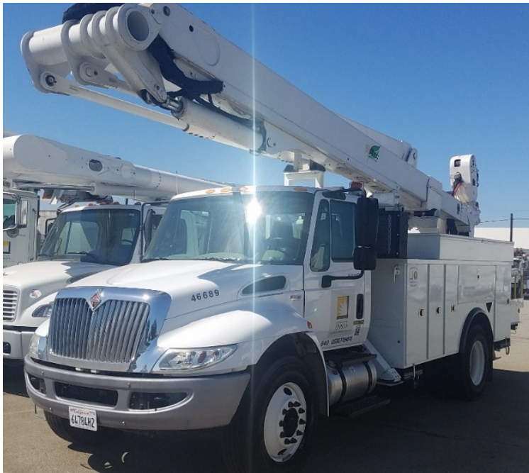
Figure 2. TA-60 Retrofitted With a Hybrid System (Medium-Duty VAPS Platform)
