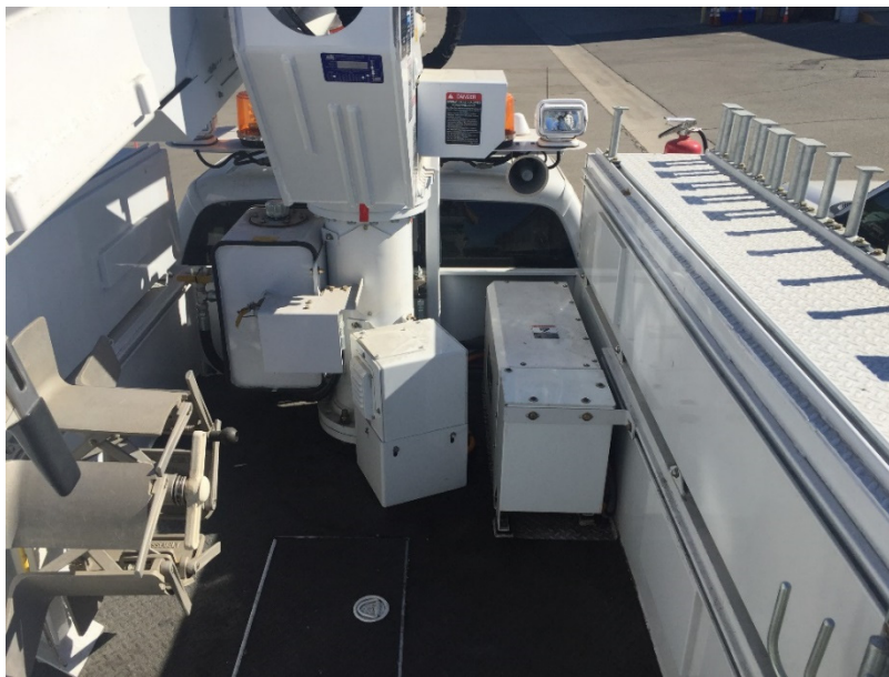
Figure 5. JEMS Components in AT-40 PHEV Test Vehicle Truck Bed
