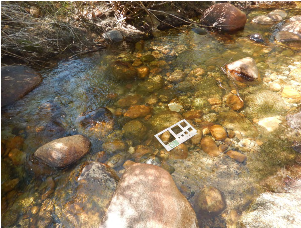
FIGURE 10. EXAMPLE SUBSTRATE AT SITE 6, TRANSECT 5, SHOWING DIVERSITY OF PARTICLE SIZES (LARGEST SQUARE IN FRAME IS 128 MM FOR REFERENCE)
