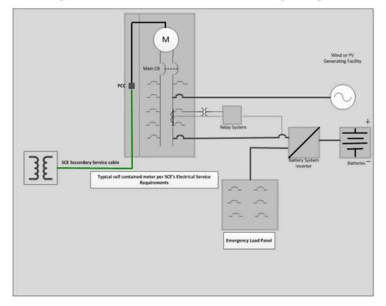
This example illustration shows the non-export relay connected and controlling the non REGF battery system. In the event that power flows (exporting) through the measurement point (Relay CT's) the relay would curtail or halt the operation of the battery system in accordance with the protection option selected by the customer.
