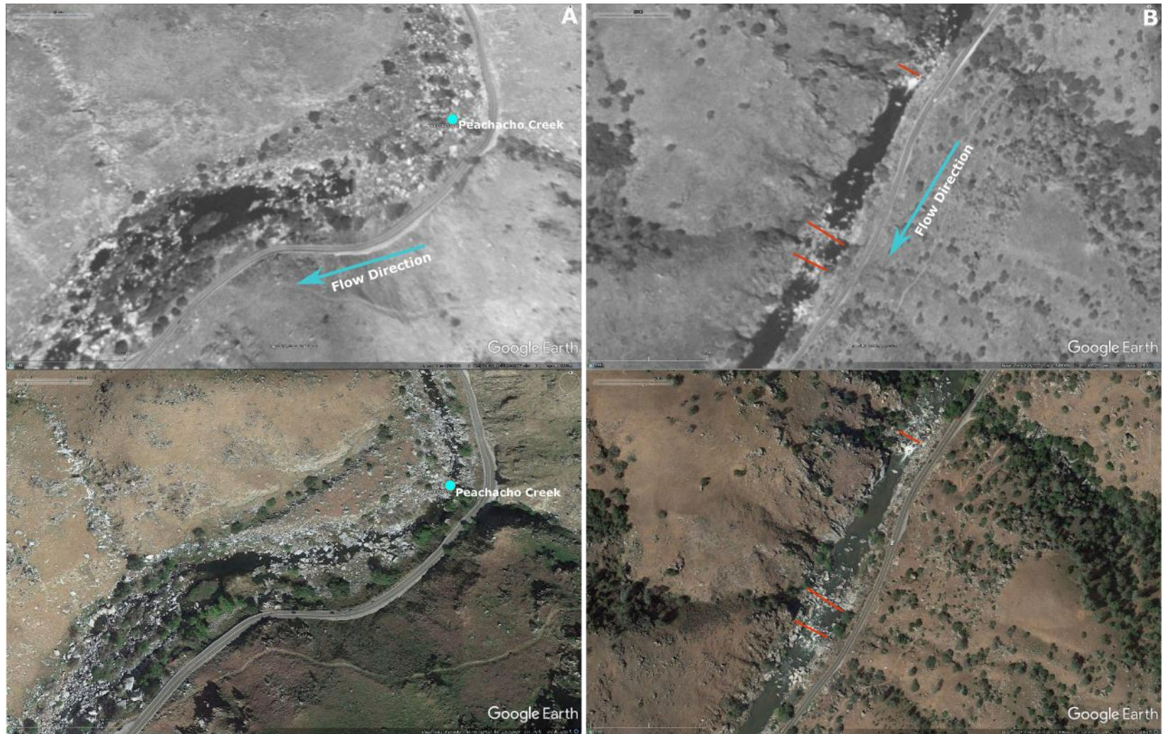
Figure 3.8-3. Representative Historical Aerial Imagery of Channel Reach Morphology in the Bypass Reach with Minimal Change Throughout the Previous License Term (1998 to Present). A) Bar morphology downstream of Peachacho Creek (RM 45.9) that shows minimal morphologic change from 2002 to 2015. B) Step-pool sequence located near RM 63 that has been maintained with minimal change from 2002 to 2013
