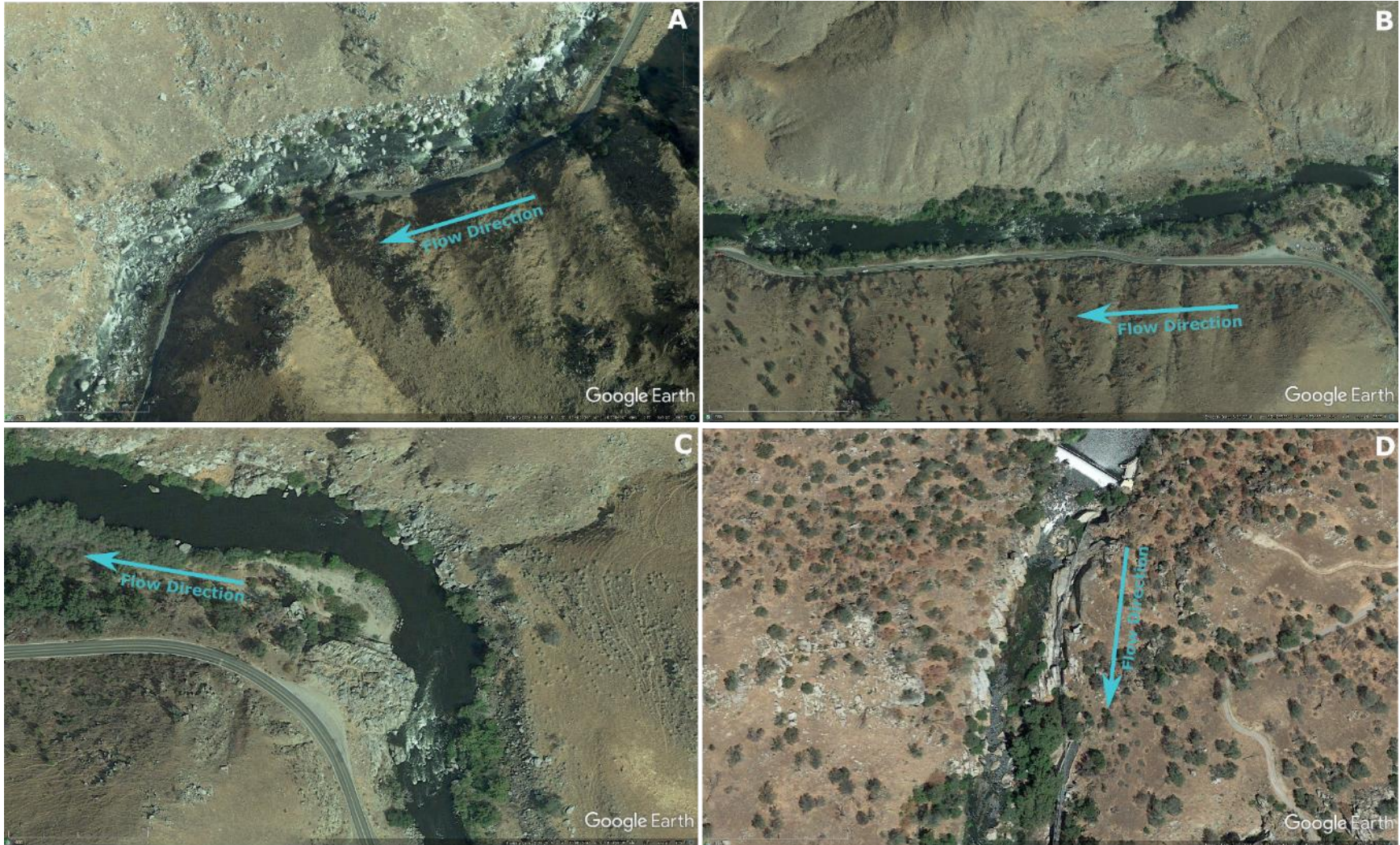
Figure 3.8-2. Representative Photographs of the A) Boulder Cascade (RM 45), B) Pool-Riffle Sequence (RM 47.5), C) Bar (RM 46.5), and D) Bedrock Channel (RM 53) Morphologies in the Bypass Reach
